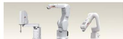
Roboter: SCARA, Knickarm, Cobots
