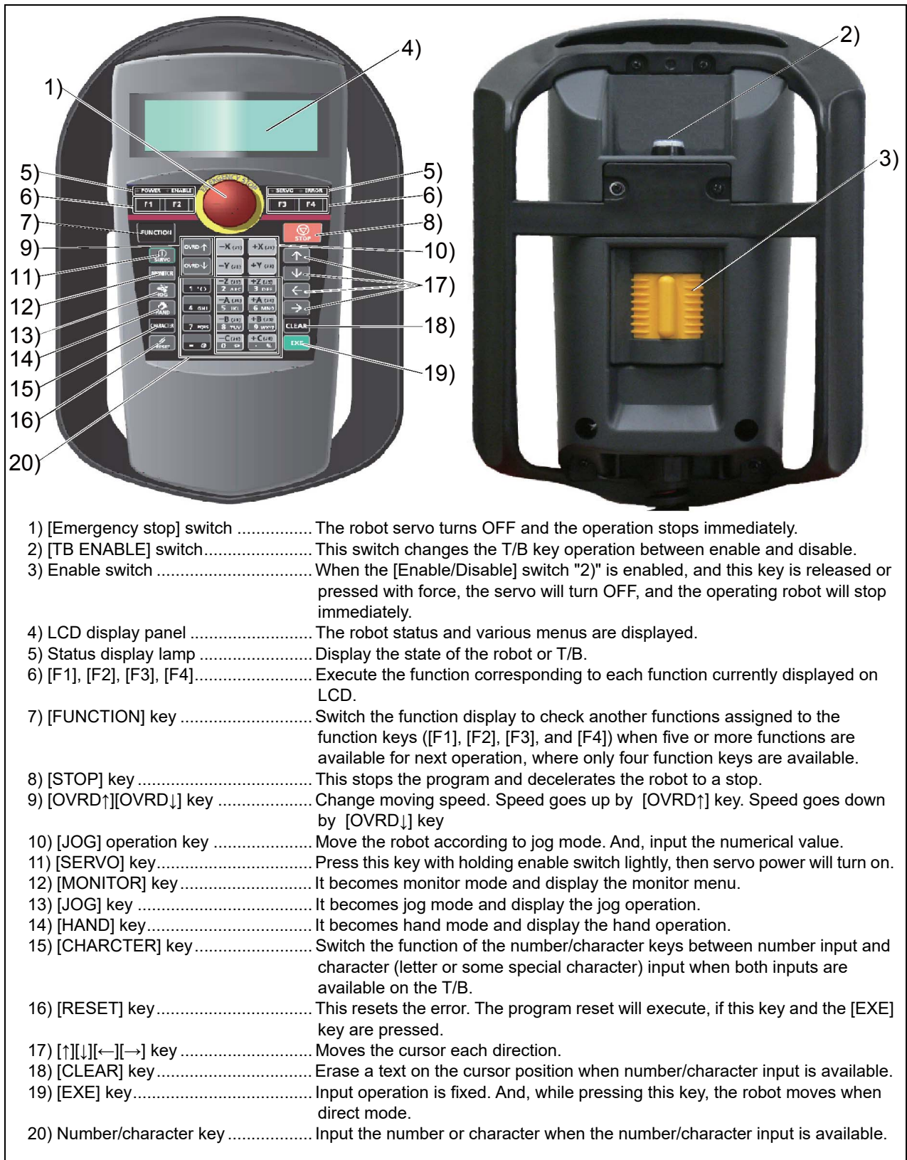
Fig.3-19: Teaching pendant key layout and main functions
