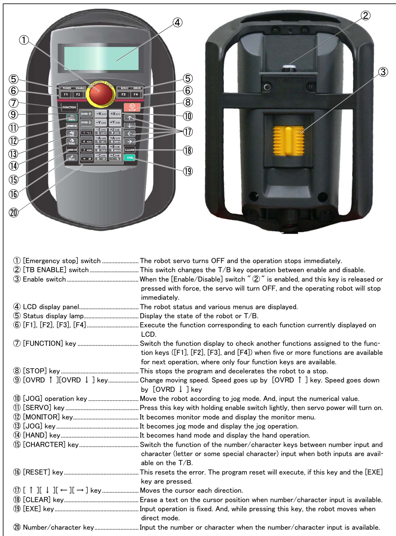
Fig.3-24 : Teaching pendant key layout and main functions
